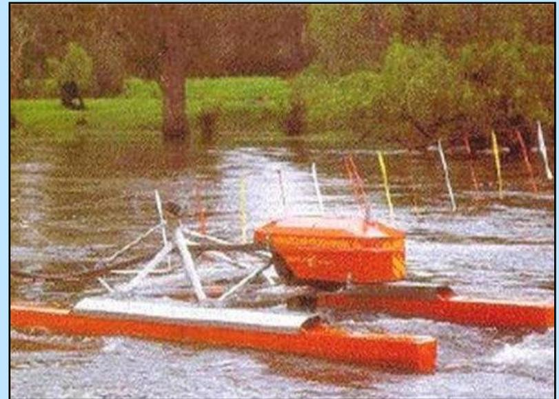
*Mounted on a floating pontoon platform and usually moored in mid-stream of a flowing river. Both rotating and reciprocating outputs are available from the gearbox. Reciprocating operates a positive displacement pump for water; Rotating drives rotating machinery to provide DC power to charge batteries directly at the riverside or AC for longer distance transmission up to 5 km.*
